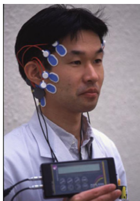
Figure 1: An overall view of portable EMG recording system.
