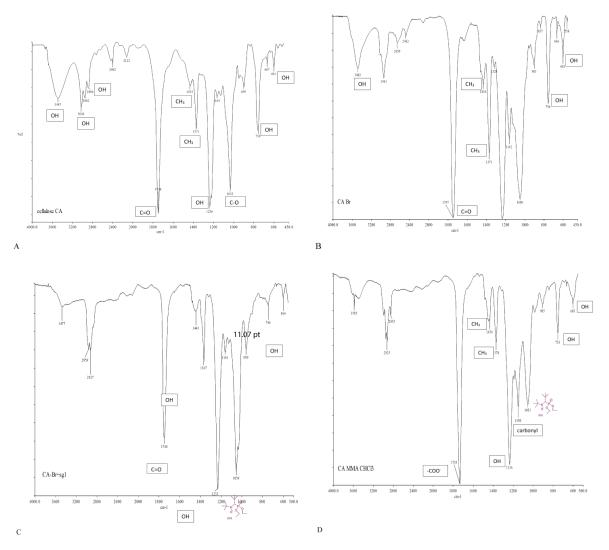
Figure 2: (A) FTIR spectra of cellulose acetate, (B) Cellulose acetate-bromide, (C) Cellulose acetate-SG1 macroalkoxyamine, (D) Cellulose acetate-copolymethyl methacrylate.
