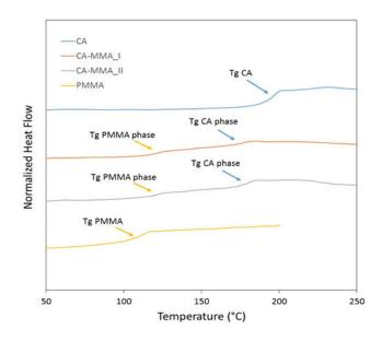
**Figure 4:** Cellulose acetate (CA), cellulose acetate-co-poly (methyl methacrylate (CA-MMA\_I) precipitated in methanol, cellulose acetate-co-poly (methyl methacrylate (CA-MMA\_II) precipitated in water.
