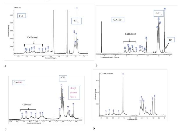
Figure 3: (A) <sup>1</sup>H NMR analyses of cellulose acetate, (B) Cellulose acetate-bromide, (C) Cellulose acetate-SG1 macroalkoxyamine, (D) Cellulose acetate-co-polymethyl methacrylate.
