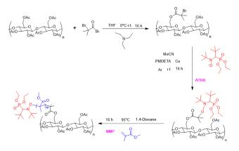
**Figure 1:** Nitoxide mediated radical polymerization of cellulose acetateco-poly (methyl methacrylate).
