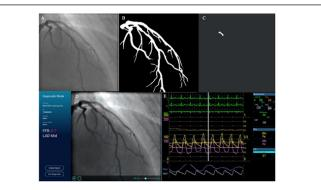
**Figure 1:** Case example of AutocathFFR. Angiographic input from the C-arm is shown in panel A, automated vessel segmentation is shown in panel B and stenosis detection in panel C. AutocathFFR output is shown in panel D indicating predicted FFR of 0.7 similar to the pressure wire based FFR shown in panel E.
