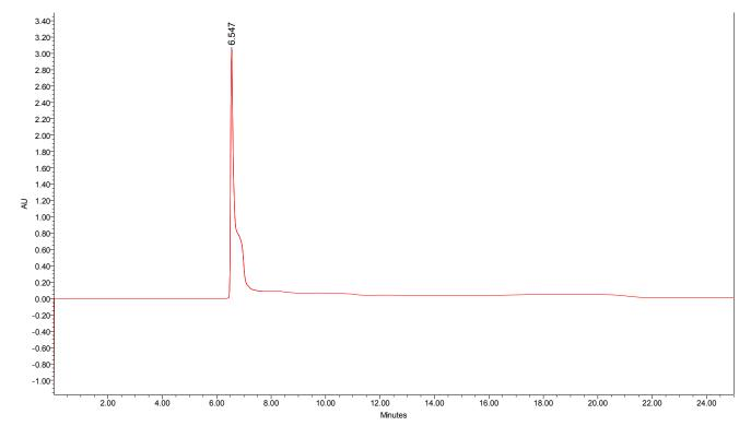
Figure 16: HPLC profile of a methanolic extract of variety D of *Piper betle*. Chromatogram of crude Sample D prepared from methanolic extract of *P.betle* L. leaf, on analytical RP-HPLC in isocratic mode using acetonitrile and water (1:1) as mobile phase and C18 column as stationary phase, at a flow rate of 0.5 ml/min. Only one peak was found at 254 nm and its retention time was 6.54 min.
