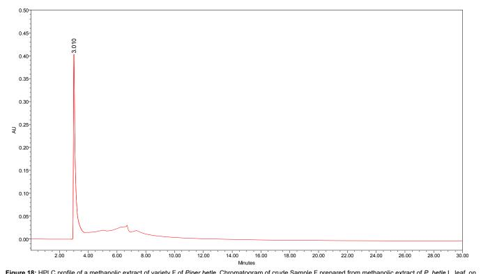
Figure 18: HPLC profile of a methanolic extract of variety F of *Piper betle*. Chromatogram of crude Sample F prepared from methanolic extract of *P. betle* L. leaf, on analytical RP-HPLC in isocratic mode using acetonitrile and water (1:1) as mobile phase and C18 column as stationary phase, at a flow rate of 0.5 ml/min. Only one peak was found at 254 nm and its retention time was 3.01 min.
