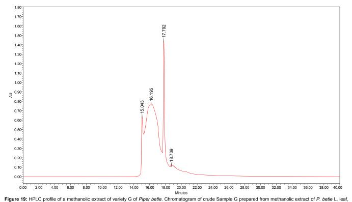
**Figure 19:** HPLC profile of a methanolic extract of variety G of *Piper betle*. Chromatogram of crude Sample G prepared from methanolic extract of *P. betle* L. leaf, on analytical RP-HPLC in isocratic mode using acetonitrile and water (1:1) as mobile phase and C18 column as stationary phase, at a flow rate of 0.5 ml/min. Four peaks were identified at 254 nm and their retention times were 15.04, 16.19, 17.79 and 18.79 min respectively.
