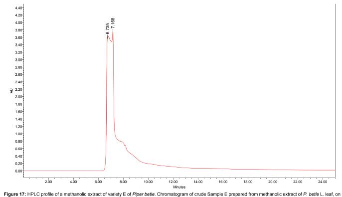
Figure 17: HPLC profile of a methanolic extract of variety E of *Piper betle*. Chromatogram of crude Sample E prepared from methanolic extract of *P. betle* L. leaf, on analytical RP-HPLC in isocratic mode using acetonitrile and water (1:1) as mobile phase and C18 column as stationary phase, at a flow rate of 0.5 ml/min. Only two peaks were found at 254 nm and their retention times were 6.73 and 7.16 min respectively.
