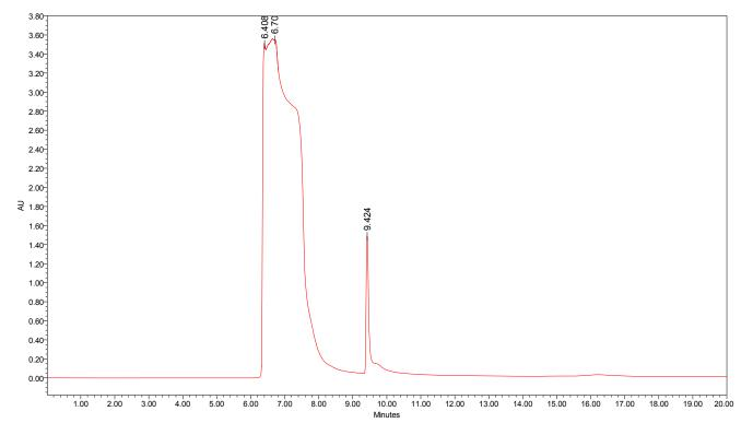
Figure 20: HPLC profile of a methanolic extract of variety H of *Piper betle*. Chromatogram of crude Sample H prepared from methanolic extract of *P. betle* L. leaf, on analytical RP-HPLC in isocratic mode using acetonitrile and water (1:1) as mobile phase and C18 column as stationary phase, at a flow rate of 0.5 ml/min. Three peaks were identified at 254 nm and their retention times were 6.40, 6.70 and 9.42 min respectively.
