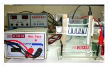
Figure 8: Small vertical gel Electrophoresis system consists of electrophoresis unit.
