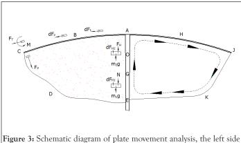
Figure 3: Schematic diagram of plate movement analysis, the left side is the force analysis diagram, and the right side is the material cycle diagram.
