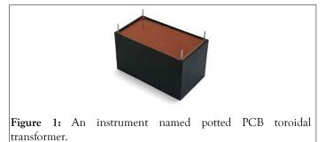
The before potting test is carried out before potting because it is difficult to rework on the transformer, in case it fails the intermediate test. After potting, the transformer is subjected to screen print marking and visual inspection. Next, the final test, called Final Quality Control (FQC) is performed on the transformer. The FQC is not as intensive as the intermediate test. Finally, the tested transformers are sent for packaging.
