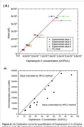
mycin C, and (B) comparison between Cephamycin C values determined by the proposed method (line) and those obtained by bioassay (dots).
