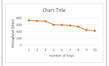
Figure 2: Throughput of TCP connection according to proposed model.
