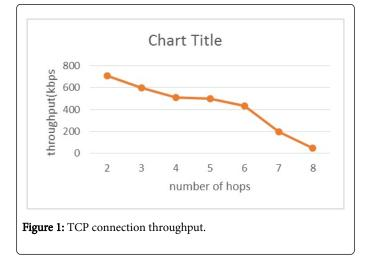
This degradation of throughput is due to false detection of packet losses as a congestion situation.
