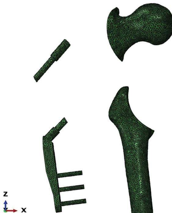
Figure 1: The separated four parts were generated for assigning isotropic heterogeneous material property of bone.
