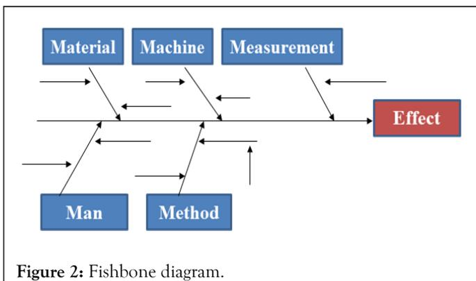
Figure 2: Fishbone diagram.
