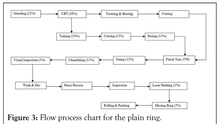
Figure 3: Flow process chart for the plain ring.
