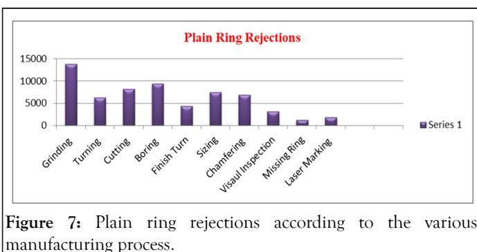
Figure 7: Plain ring rejections according to the various manufacturing process.
