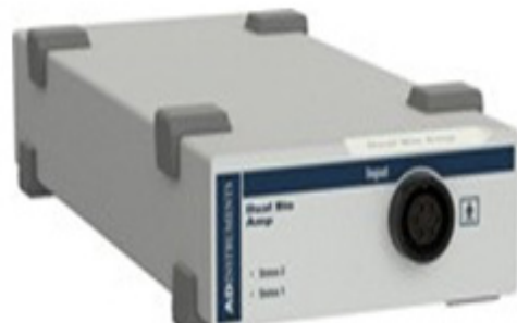
Figure 3: Dual bio amp DB066 device in power lab 8/30 (image by AD Instrument and reproduced with permission).
