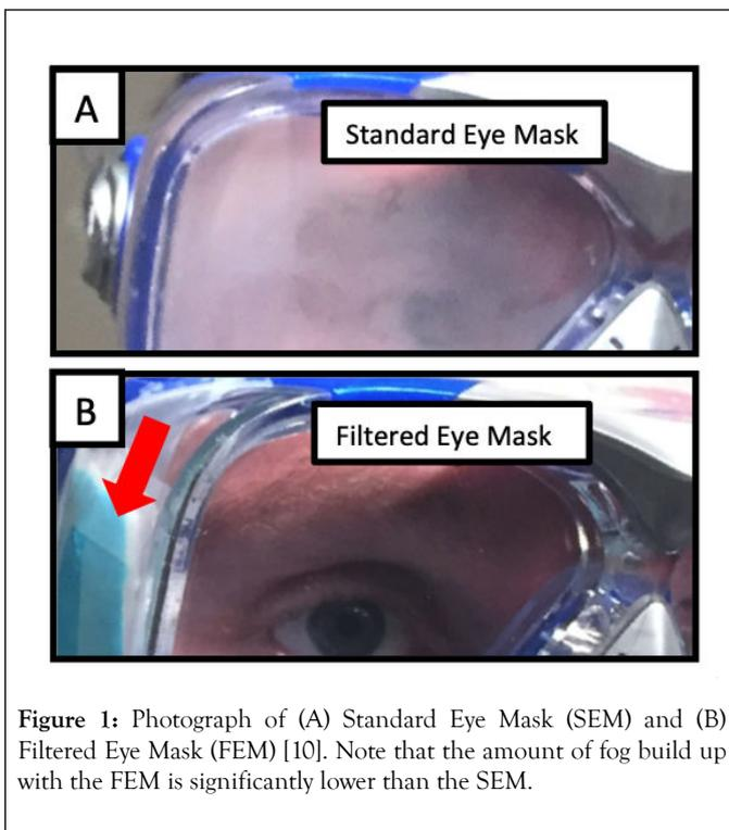
**Figure 1:** Photograph of (A) Standard Eye Mask (SEM) and (B) Filtered Eye Mask (FEM) [10]. Note that the amount of fog build up with the FEM is significantly lower than the SEM.
