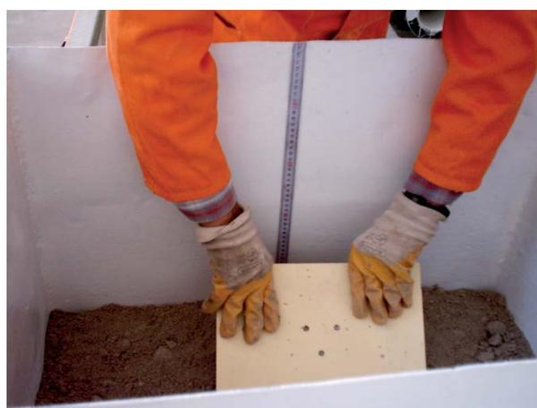
Figure 3: Compaction procedure.
