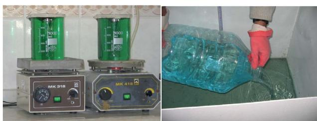
Figure 5: Preparation procedure and addition of Cu and Cr solutions into the sections.
