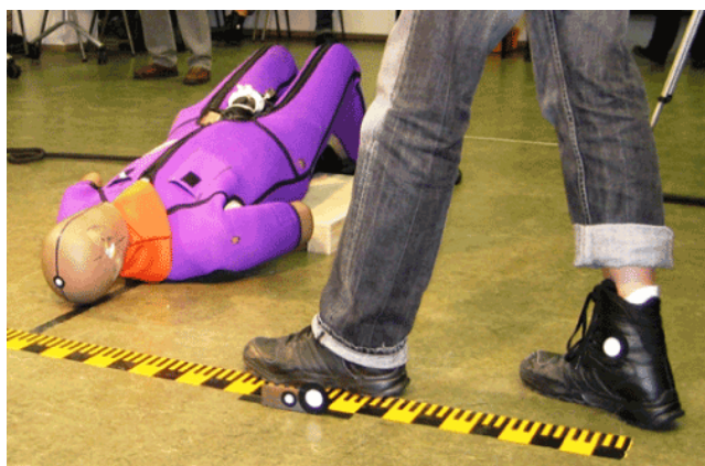
Figure 3: Study Part B/C: Set up for horizontal kick test: the crash-dummy was lying in supine position, while the kick was performed laterally to the body.
