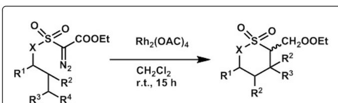
**Scheme 4:** Formation of six-membered cyclic sulfones by C-H insertion.
