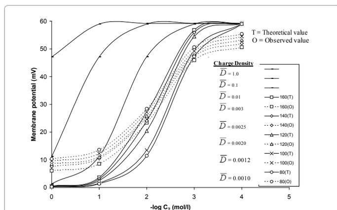
Figure 2: Plots of membrane potentials versus  $-\log C_2$  at different concentrations of NaCl electrolyte solution for composite membranes prepared at different pressures 80-160 MPa.
