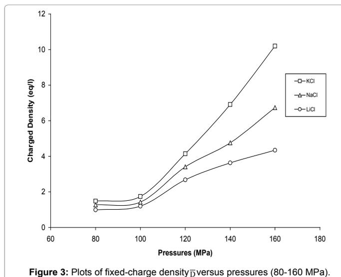
Figure 3: Plots of fixed-charge density  $\bar{D}$  versus pressures (80-160 MPa).
