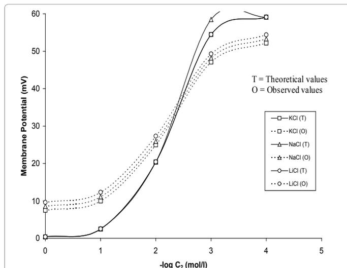
**Figure 6:** Membrane potentials across composite membranes using various electrolyte (1:1) solutions at different concentrations.
