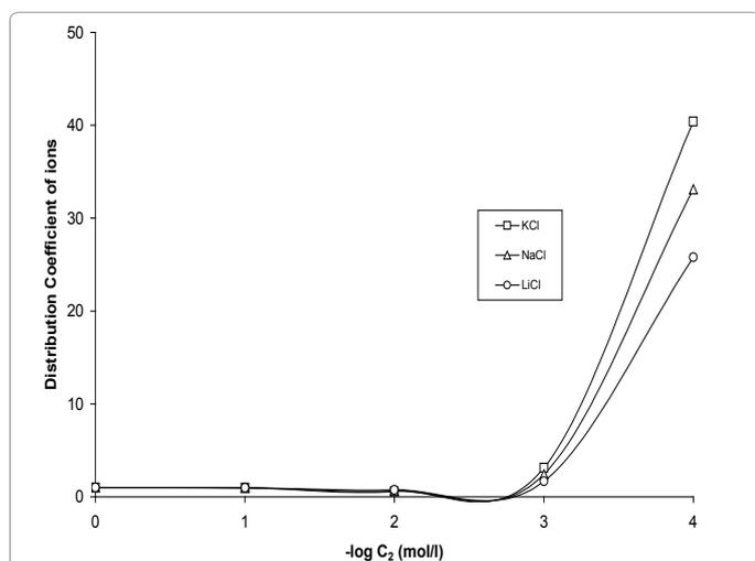
Figure 4: Plots of Distribution coefficient of ions ( $K_{\pm}$ ) versus  $-\log C_2$  (mol/l).
