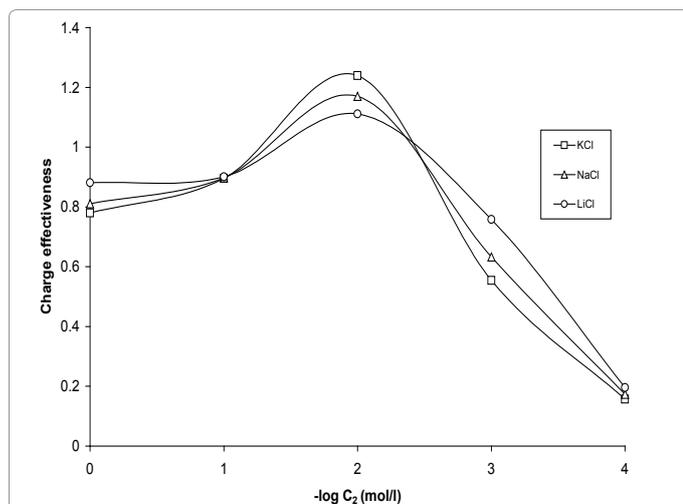
**Figure 5:** Plots of Charge effectiveness versus  $-\log C_2$  (mol/l) for 1:1 electrolyte at different concentrations.
