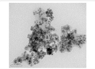
Figure 2: Fe<sub>3</sub>O<sub>4</sub>@C core-shell nanoparticles consist of a magnetic core and carbon coating.
