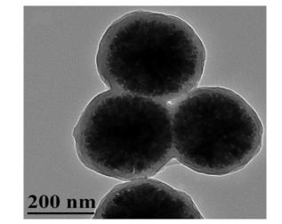
Figure 3: Fe\_{\_3}O\_{\_4}@C core-shell nanoparticles consist of a magnetic core and carbon coating.
