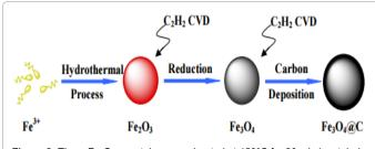
Figure 8: The  $\alpha$ -Fe\_2O\_3 nanotubes were heated at 450°C for 30 min in a tubular furnace under a  $N_2:C_2H_2$  flow.
