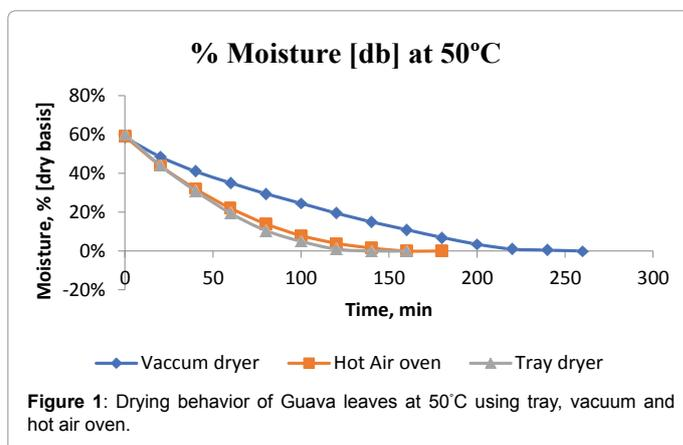
Figure 1: Drying behavior of Guava leaves at 50°C using tray, vacuum and hot air oven.
