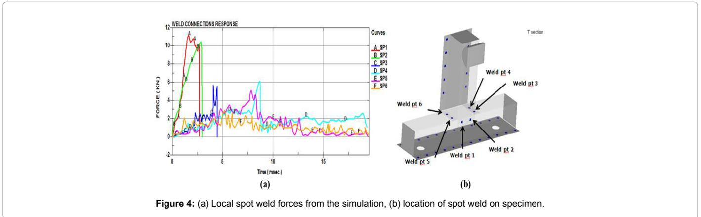
Figure 4: (a) Local spot weld forces from the simulation, (b) location of spot weld on specimen.
