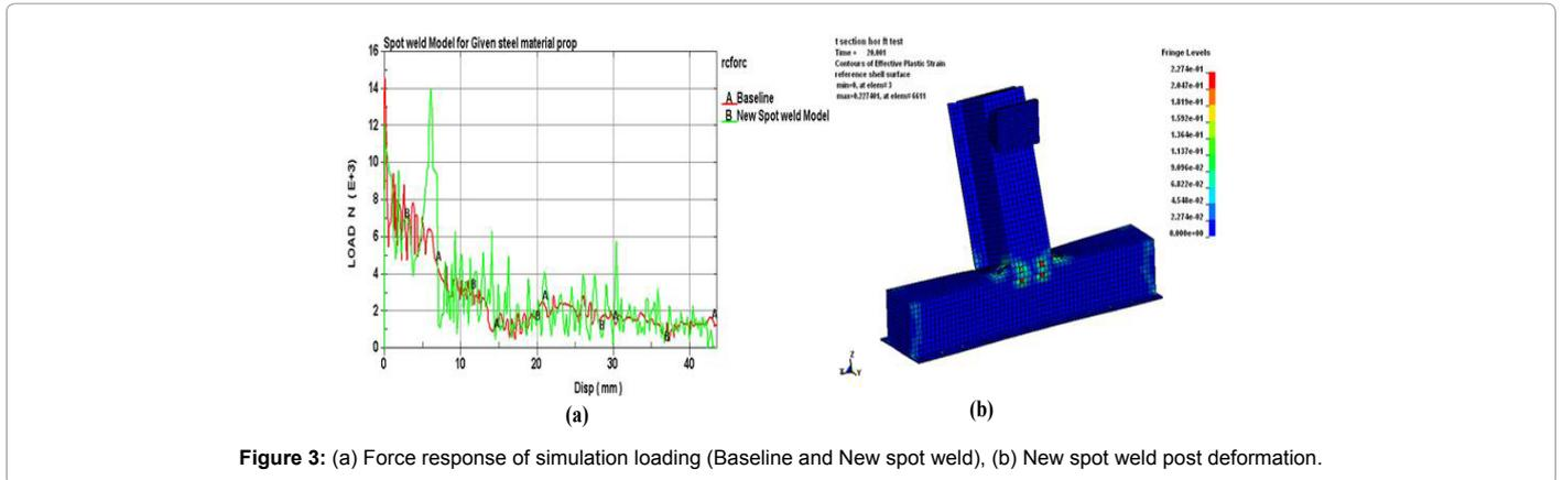
Figure 3: (a) Force response of simulation loading (Baseline and New spot weld), (b) New spot weld post deformation.
