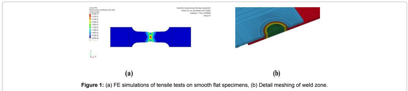
Figure 1: (a) FE simulations of tensile tests on smooth flat specimens, (b) Detail meshing of weld zone.
