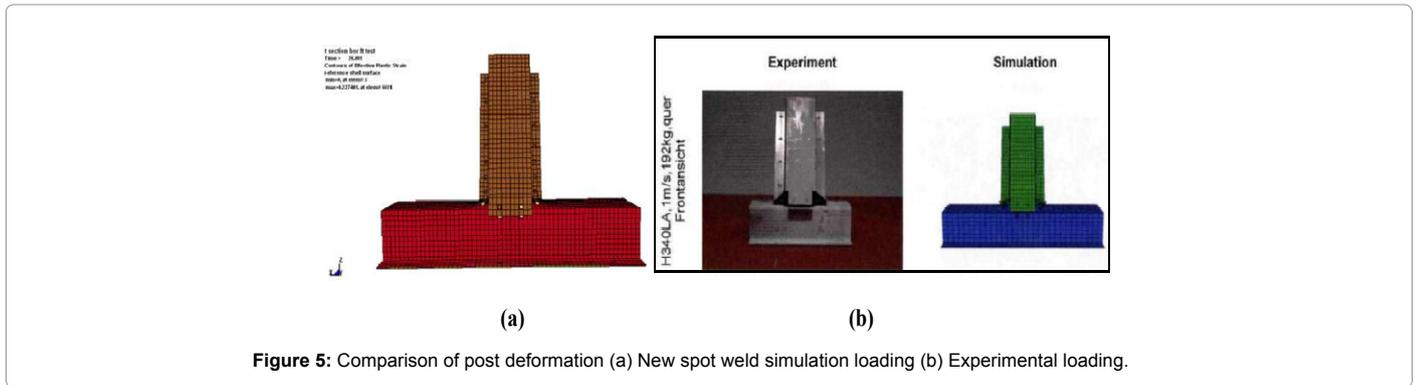
Figure 5: Comparison of post deformation (a) New spot weld simulation loading (b) Experimental loading.
