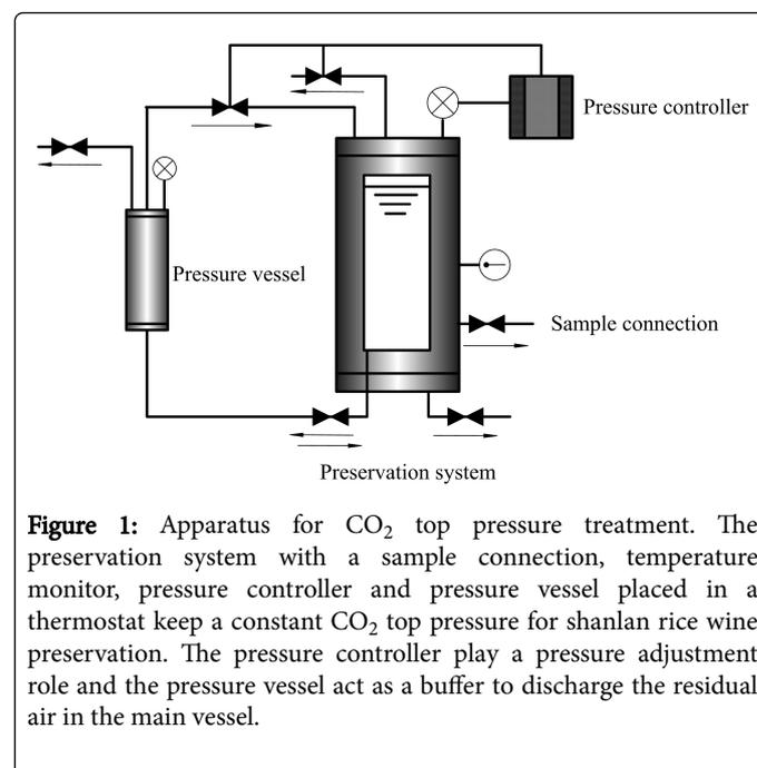
**Figure 1:** Apparatus for CO<sub>2</sub> top pressure treatment. The preservation system with a sample connection, temperature monitor, pressure controller and pressure vessel placed in a thermostat keep a constant CO<sub>2</sub> top pressure for shanlan rice wine preservation. The pressure controller play a pressure adjustment role and the pressure vessel act as a buffer to discharge the residual air in the main vessel.
