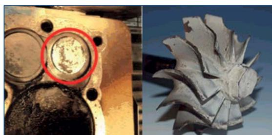
**Figure 2:** Incrustation on valves and turbines.
