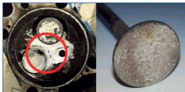
**Figure 1:** Deposits on the generator valves.
