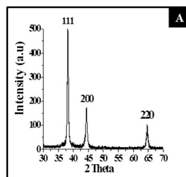
Figure 2: The powder X-ray diffraction of gold nanostructures.
