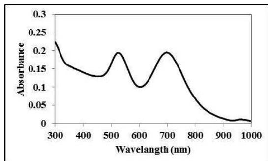
Figure 3: The Absorbance spectra of gold nanostructures.
