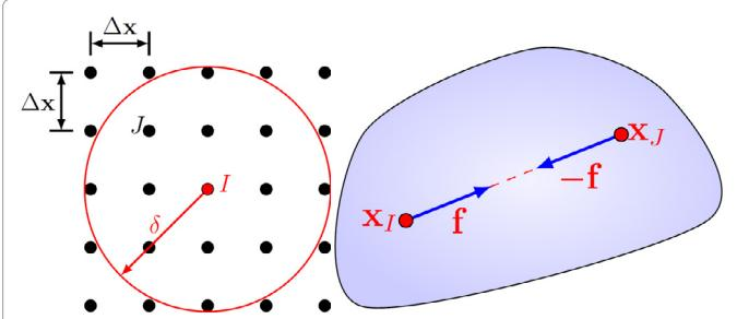
Figure 1: Peridynamic model: Discretization, horizon and pairwise forces.
