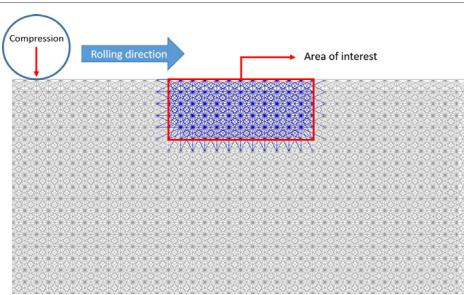
Figure 2: The bond-based peri-dynamic model under rolling contact.
