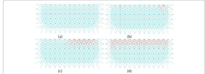
Figure 3: Crack initiation and propagation at: (a)  $N=6000$  cycles; (b)  $N=89000$  cycles; (c)  $N=150000$  cycles; and (d)  $N=350000$  cycles.
