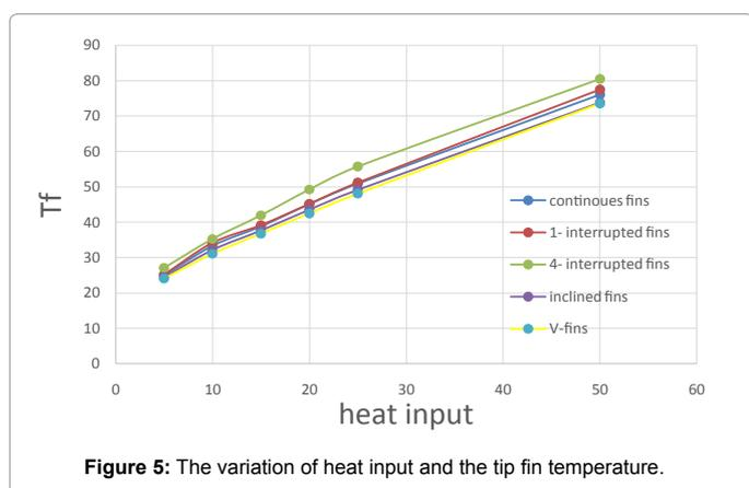
Average Nusselt numbers decrease with increasing the finning factor for same heat input, in this case must V-fin the lowest but heat transfer coefficient depended also on configuration of air flow.
