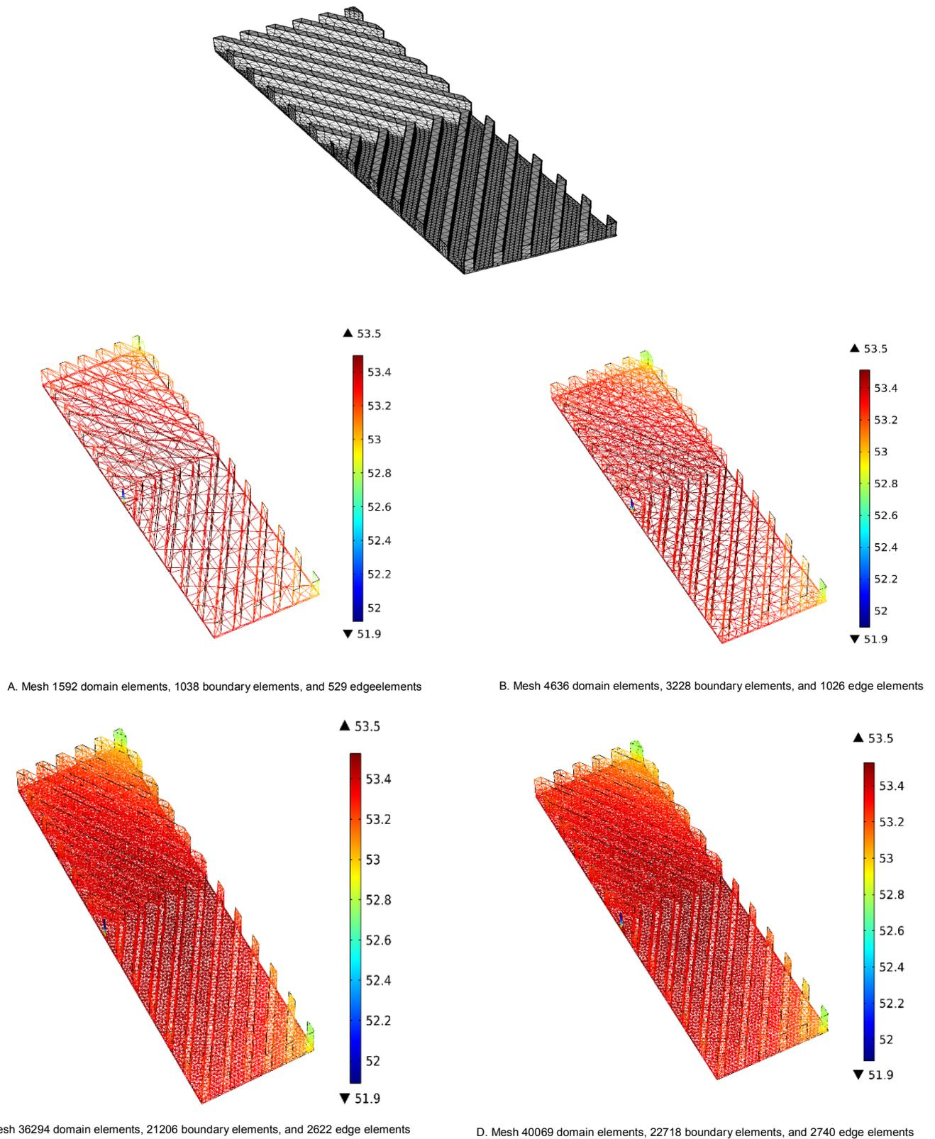
Figure 2: Mesh independence of V-fin.
