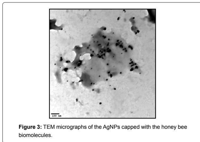
Figure 3: TEM micrographs of the AgNPs capped with the honey bee biomolecules.
