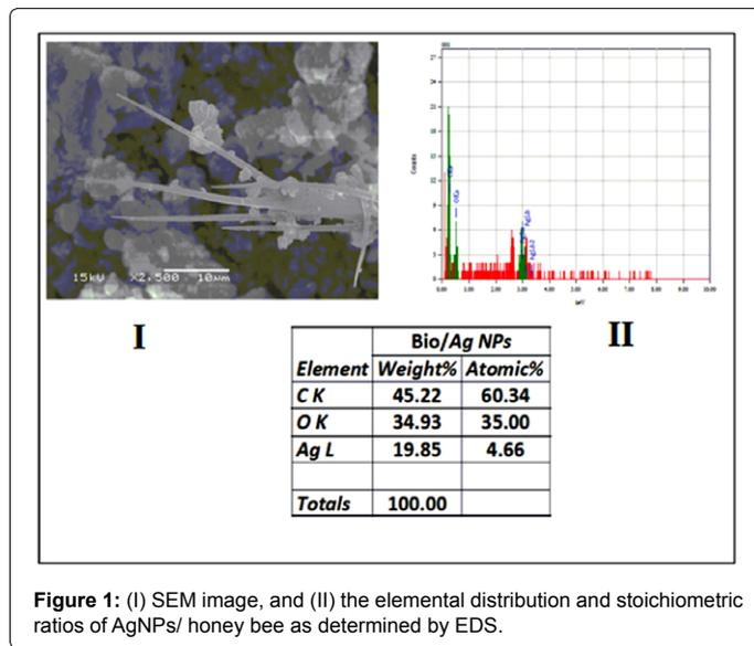
Figure 1: (I) SEM image, and (II) the elemental distribution and stoichiometric ratios of AgNPs/ honey bee as determined by EDS.
