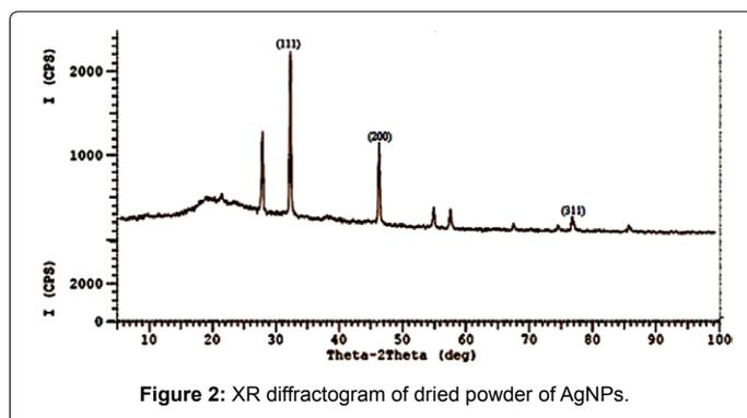
Figure 2: XR diffractogram of dried powder of AgNPs.
