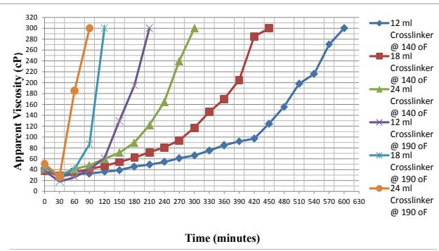
Figure 2: Viscosity build-up for 5% KCL water-shutoff design.
