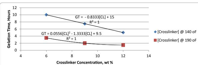
**Figure 8:** Effect of cross-linker concentration on gelation time for 5% KCl.
