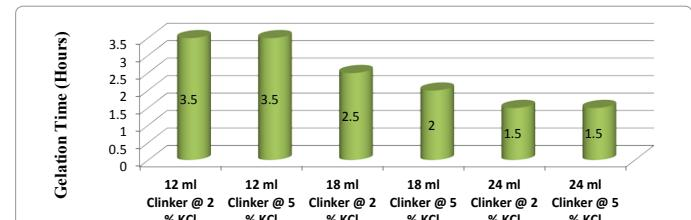
**Figure 6:** Effect of brine on gelation time for water-shutoff design @ 190°F.
