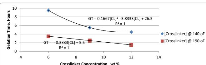
**Figure 7:** Effect of cross-linker concentration on gelation Time for 2% KCl.
