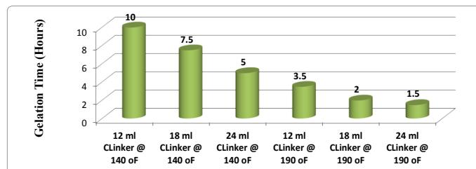
**Figure 4:** Temperature and crosslinker effect on gel time of water-shutoff for 5% KCl.
