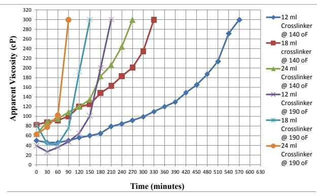
Figure 1: Viscosity build-up for 2% KCl water-shutoff design.
