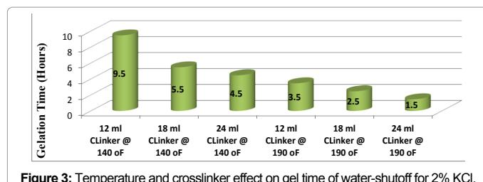
**Figure 3:** Temperature and crosslinker effect on gel time of water-shutoff for 2% KCl.
