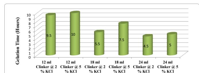
**Figure 5:** Effect of brine on gelation time for water-shutoff design @ 140°F.
