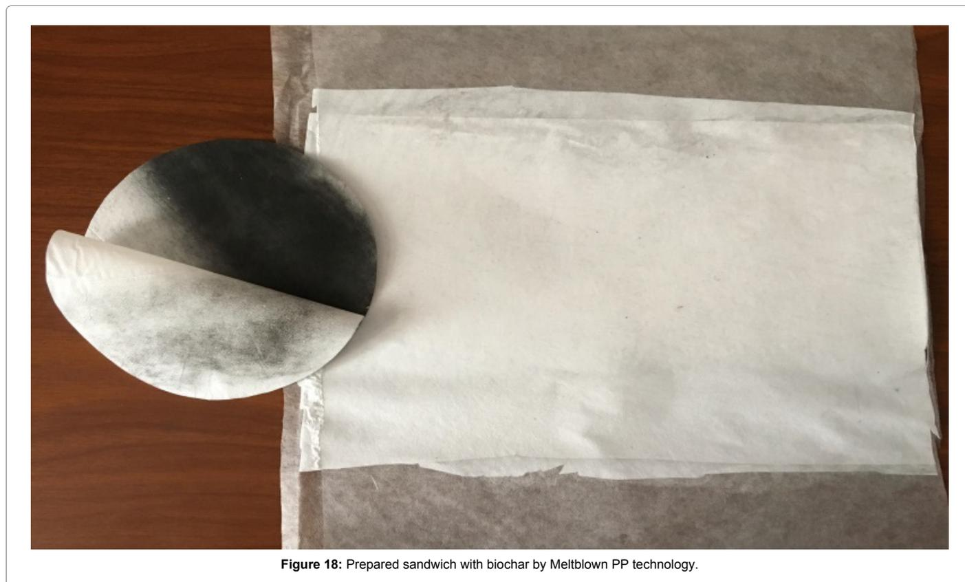
Figure 18: Prepared sandwich with biochar by Meltblown PP technology.
