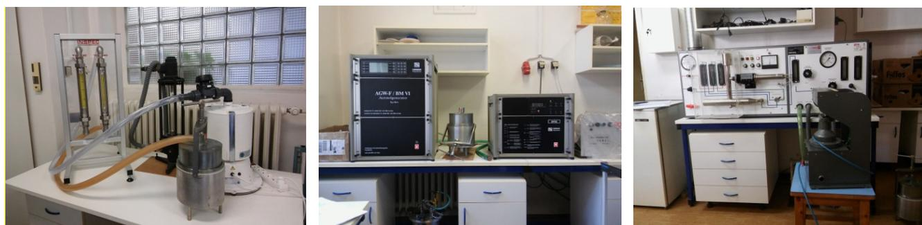
Figure 19: Measurement device for respiratory resistance and aerosol penetration for NaCl and paraffin oil (a) Sodium chloride test - Breakthrough of NaCl after 3 minutes. Flow rate 45 l/min.
