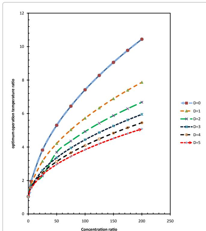
Figure 3: Dependence of the optimum operating temperature ratio on the engine parameters and the concentration ratio of the solar collector.
