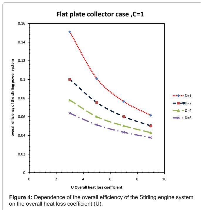
Figure 4: Dependence of the overall efficiency of the Stirling engine system on the overall heat loss coefficient (U).
