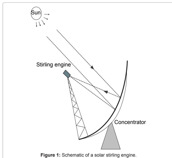
Figure 1: Schematic of a solar Stirling engine.
