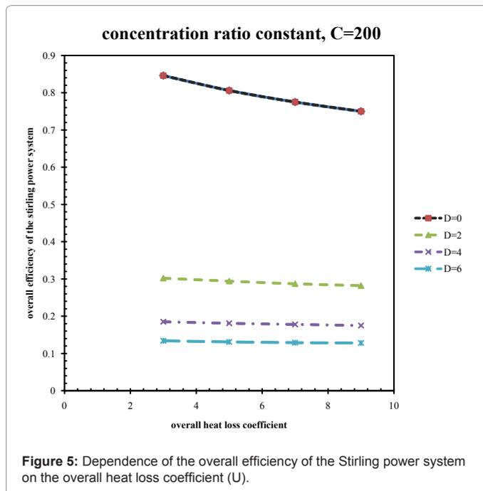
Figure 5: Dependence of the overall efficiency of the Stirling power system on the overall heat loss coefficient (U).
