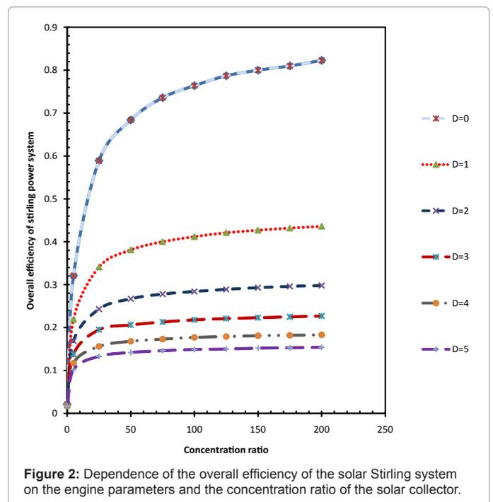
Figure 2: Dependence of the overall efficiency of the solar Stirling system on the engine parameters and the concentration ratio of the solar collector.
