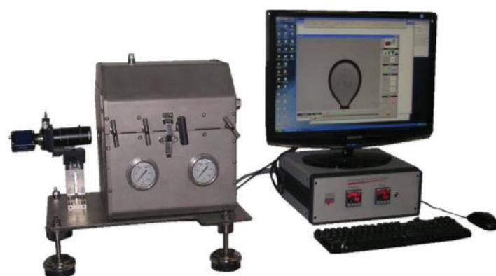
Figure 1: IFT-700 Apparatus.
