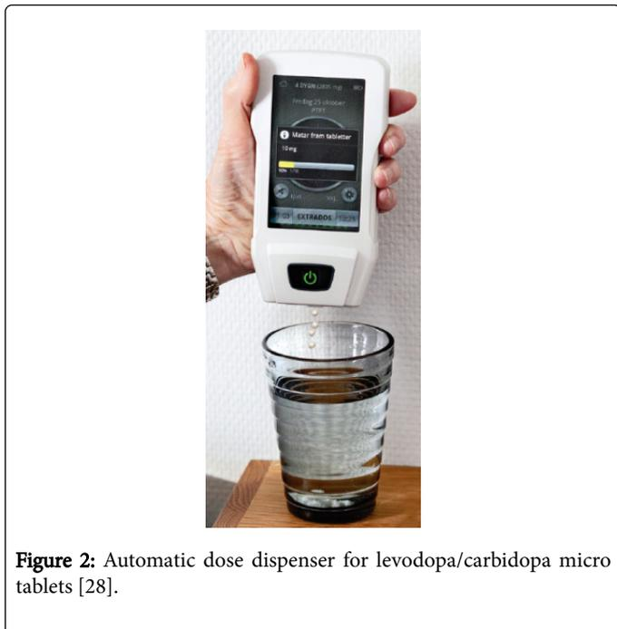
**Figure 2:** Automatic dose dispenser for levodopa/carbidopa micro tablets [28].
