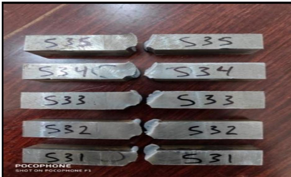
Figure 2: Impact specimens after the test.
