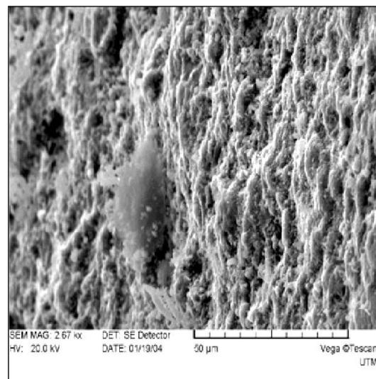
Figure 2. Surface processed by anode oxidation
