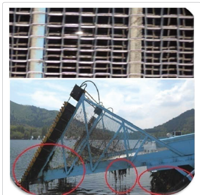
Figure 3: The perforated plates of harvester as well as loading vehicle provide an escape route for invertebrates and plant propagules like turion and buds. The macrophytes attached to harvester head aid in dispersion of viable propagules as the machine moves through water.
