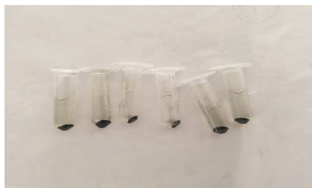
Figure 2: Black pellets sedimented during centrifugation showing the synthesis of iron nanoparticles.
