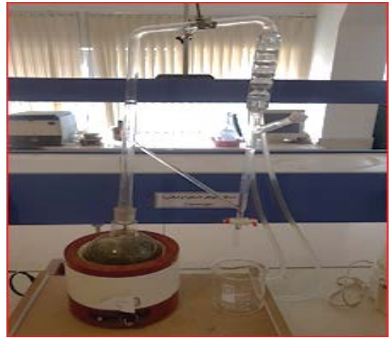
Figure 5: Essential oil preparation by Clevenger machine.
