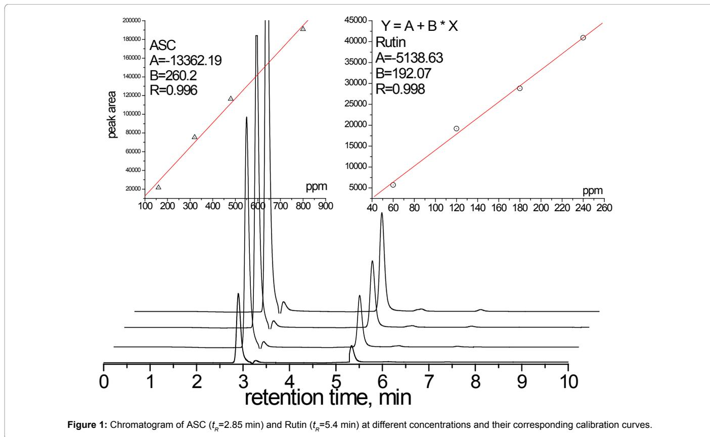
Figure 1: Chromatogram of ASC ( $t_R=2.85$  min) and Rutin ( $t_R=5.4$  min) at different concentrations and their corresponding calibration curves.
