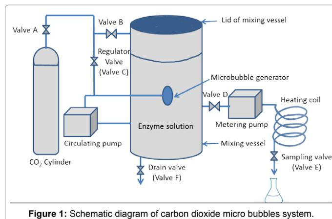
Figure 1: Schematic diagram of carbon dioxide micro bubbles system.
