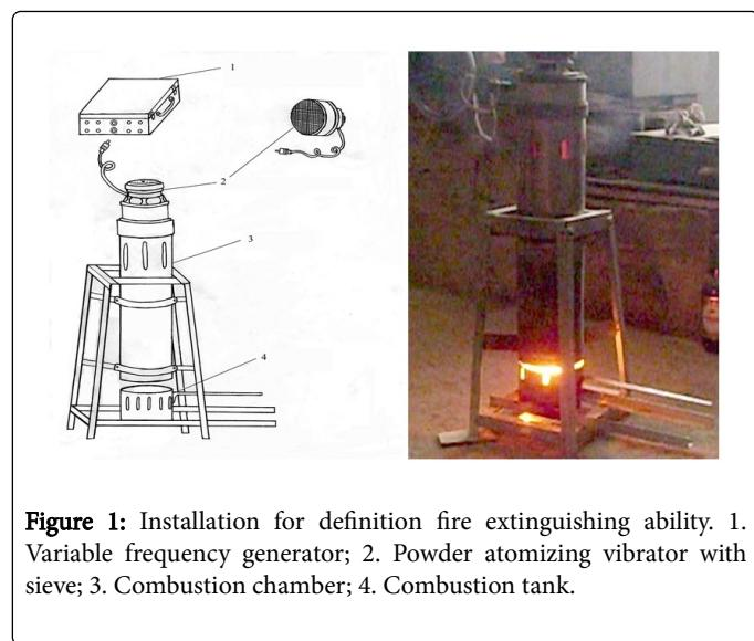
**Figure 1:** Installation for definition fire extinguishing ability. 1. Variable frequency generator; 2. Powder atomizing vibrator with sieve; 3. Combustion chamber; 4. Combustion tank.
