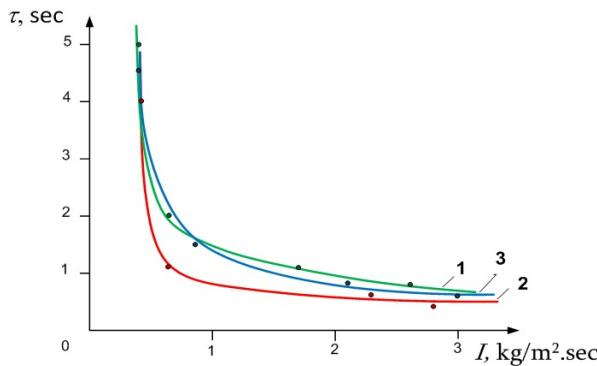
**Figure 2:** The relation of extinguish time on powder supply intensity.
