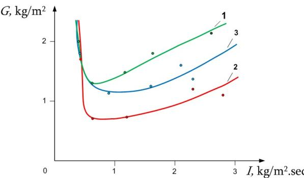
**Figure 3:** The relation of powder specific consumption on supply intensity.
