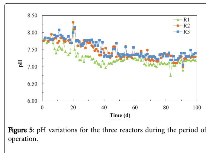
Figure 5: pH variations for the three reactors during the period of operation.
