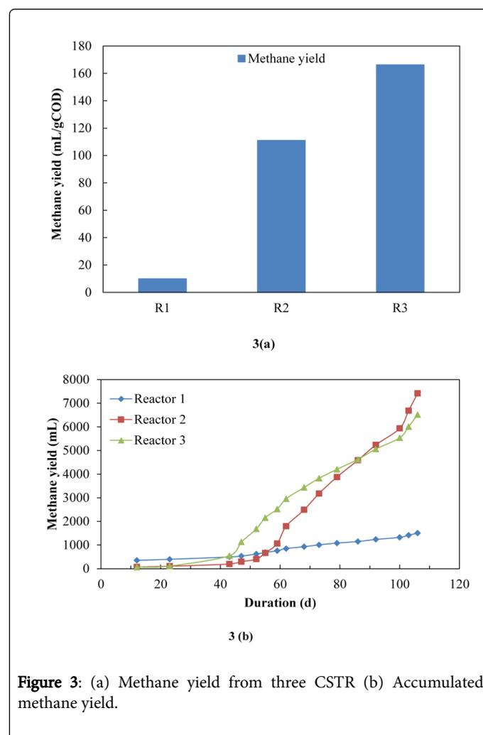
**Figure 3:** (a) Methane yield from three CSTR (b) Accumulated methane yield.
