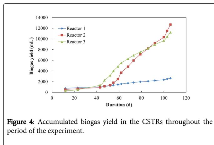
Figure 4: Accumulated biogas yield in the CSTRs throughout the period of the experiment.
