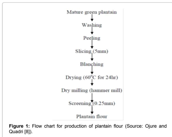
Figure 1: Flow chart for production of plantain flour (Source: Ojure and Quadri [8]).
