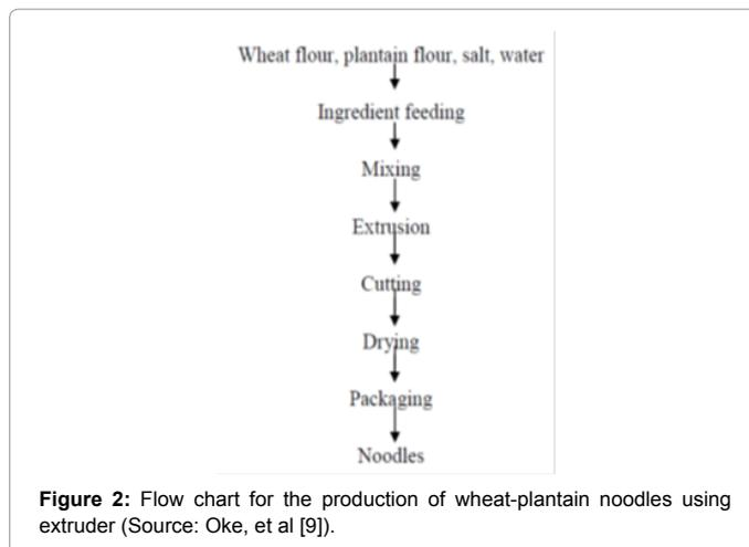
Figure 2: Flow chart for the production of wheat-plantain noodles using extruder (Source: Oke, et al [9]).
