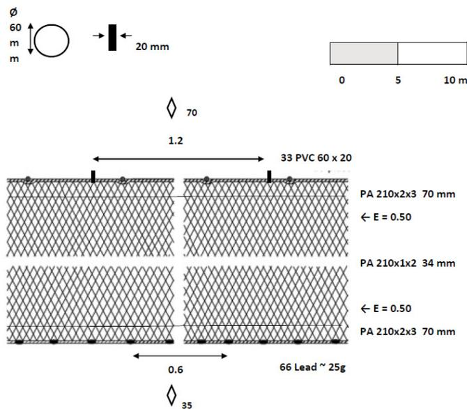
Figure 2b: Design of multifilament shrimp gill net.
