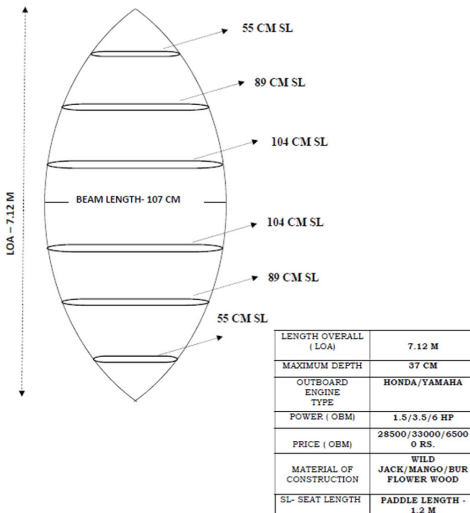
Figure 4: Technical specification of traditional wooden canoe.
