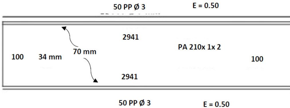
Figure 2a: Design of multifilament shrimp gill net.
