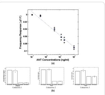
Figure 3: (a) Frequency response of NMR sensors as a function of ANT concentrations. Every data point on this plot represents an average of output signals obtained in multiple experiments done with different NMR, whereas the range of output signals obtained from these experiments is shown as the error bar. (b) Evaluation of unknown protein cocktails 1, 2, and 3 comparing the measured values with the actual, as-prepared values. Error bars represent the 95% confidence interval; n = 4 trials
