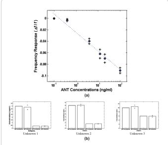
**Figure 3:** (a) Frequency response of NMR sensors as a function of ANT concentrations. Every data point on this plot represents an average of output signals obtained in multiple experiments done with different NMR, whereas the range of output signals obtained from these experiments is shown as the error bar. (b) Evaluation of unknown protein cocktails 1, 2, and 3 comparing the measured values with the actual, as-prepared values. Error bars represent the 95% confidence interval; n=4 trials
