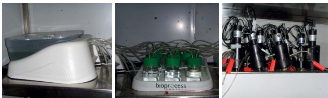
Figure 1: The bio process reactor used for the BMP test (a) Flow cells that transmit data (b) NaOH trap CO_2 (c) AMPTS II.
