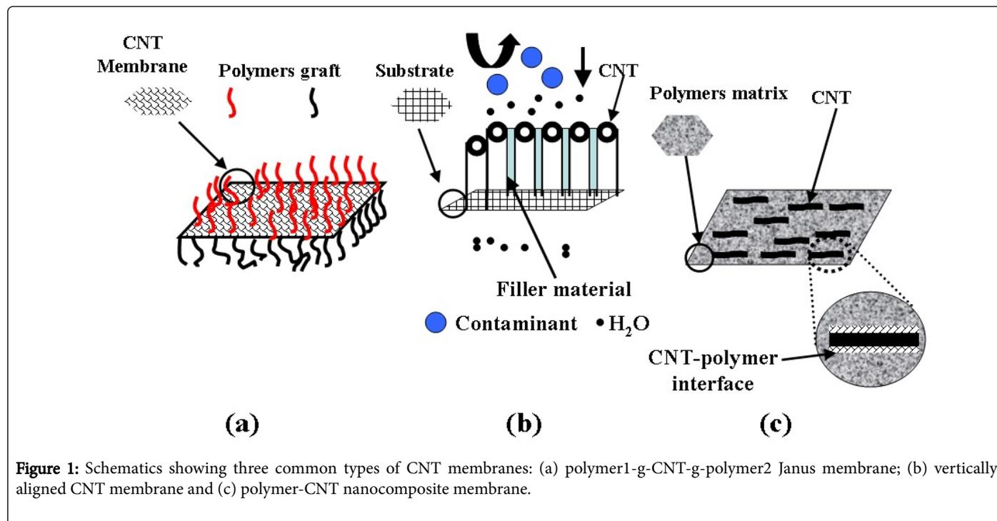
**Figure 1:** Schematics showing three common types of CNT membranes: (a) polymer1-g-CNT-g-polymer2 Janus membrane; (b) vertically aligned CNT membrane and (c) polymer-CNT nanocomposite membrane.
