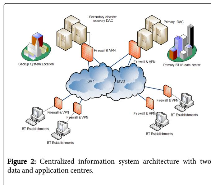
Figure 2: Centralized information system architecture with two data and application centres.
