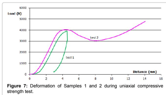
Figure 7: Deformation of Samples 1 and 2 during uniaxial compressive strength test.
