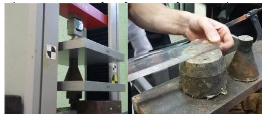
Figure 6: Uniaxial compressive strength test of the clog.
