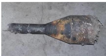
Figure 5: Stopper clog removed from the machine when the frame was cleaned.
