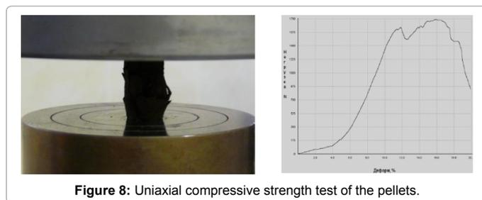
Figure 8: Uniaxial compressive strength test of the pellets.
