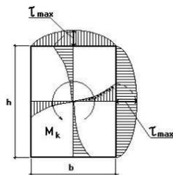
Figure 3: Curve showing shaft moment of resistance with auger narrowing, h=115 mm, b=113.
