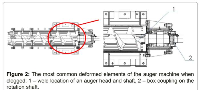
**Figure 2:** The most common deformed elements of the auger machine when clogged: 1 – weld location of an auger head and shaft, 2 – box coupling on the rotation shaft.
