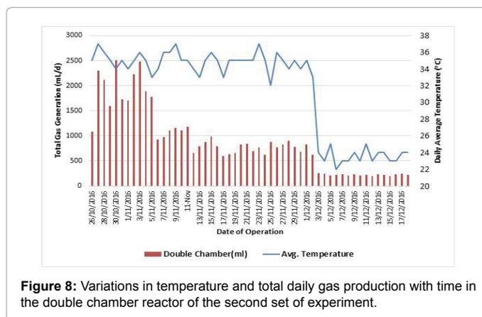
Figure 8: Variations in temperature and total daily gas production with time in the double chamber reactor of the second set of experiment.
