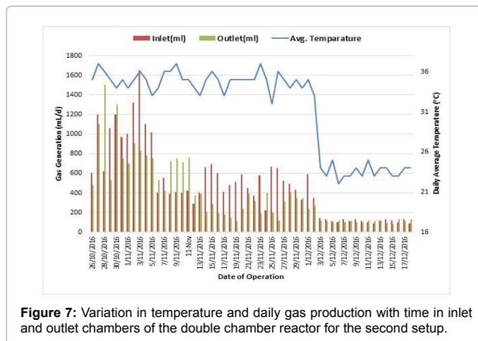
Figure 7: Variation in temperature and daily gas production with time in inlet and outlet chambers of the double chamber reactor for the second setup.
