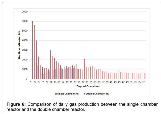
Figure 6: Comparison of daily gas production between the single chamber reactor and the double chamber reactor.
