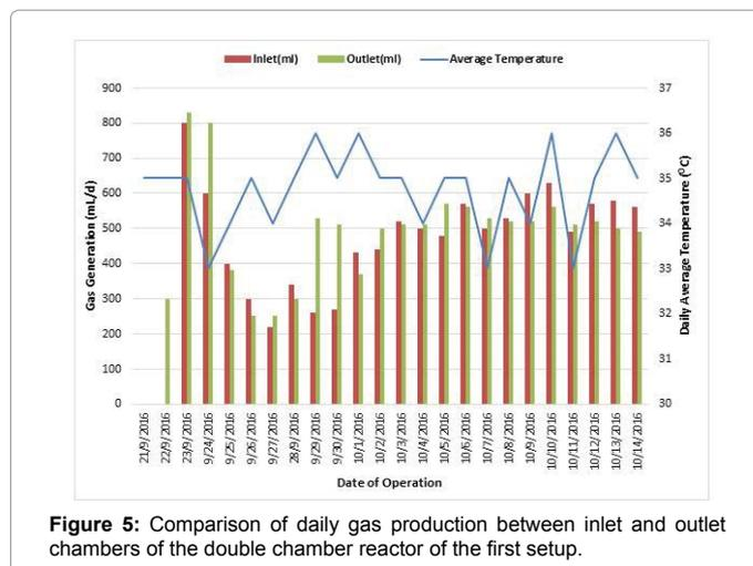
Figure 5: Comparison of daily gas production between inlet and outlet chambers of the double chamber reactor of the first setup.
