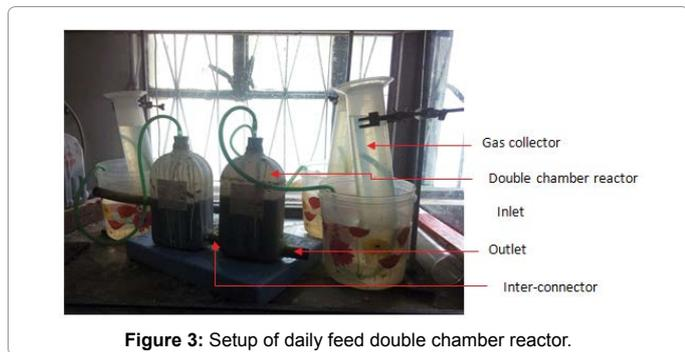
Figure 3: Setup of daily feed double chamber reactor.
