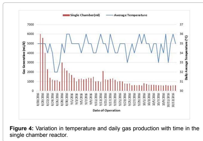
Figure 4: Variation in temperature and daily gas production with time in the single chamber reactor.
