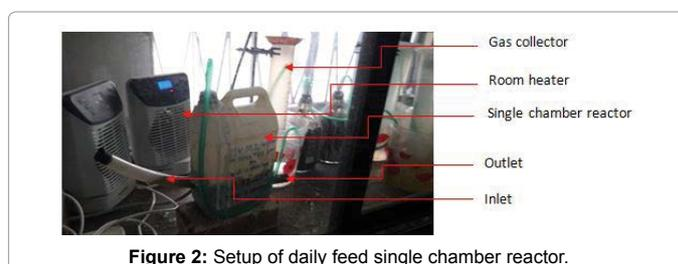
Figure 2: Setup of daily feed single chamber reactor.
