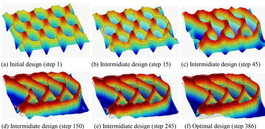
Figure 3: Level-set surfaces of a cantilever beam.
