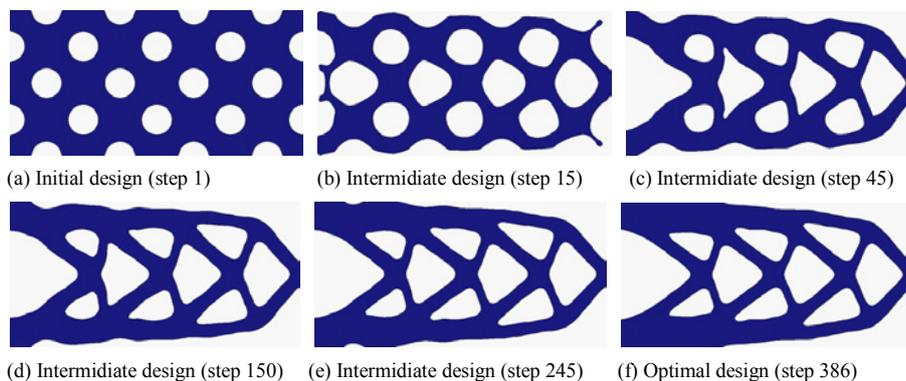
Figure 2: Level-set contours of a cantilever beam.
