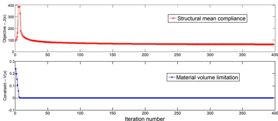
Figure 4: Convergence of the objective function and the volume constraint.
