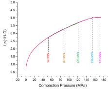
Ibuprofen Heckel transformation at varying compaction pressures.
