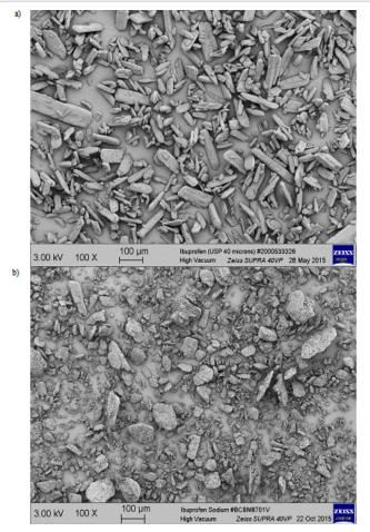
Figure 1: Electronmicrograph showing a) ibuprofen (x100) and b) ibuprofen sodium (x100).
