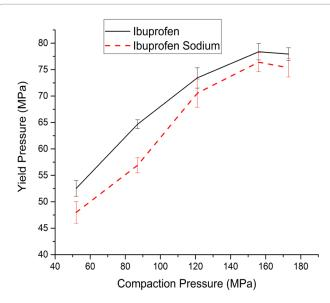
**Figure 6:** Effect of compaction pressure on yield for ibuprofen and ibuprofen sodium.
