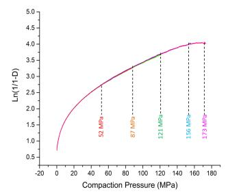
Figure 4: Heckel transformations of ibuprofen at varying compaction pressures.
