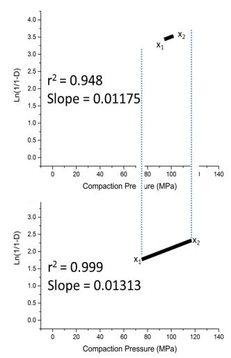
**Figure 3:** An example of the extension of the linear range of the Heckel model in order to achieve the highest regression coefficient.
